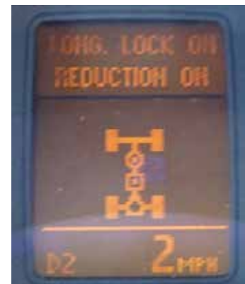
The Cayenne display that confirms low-range and differential locking for safe beach driving
